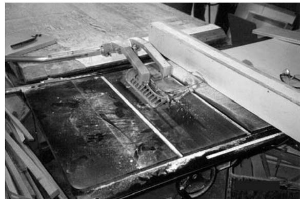
Table saw equipped with self-adjusting blade guard.
