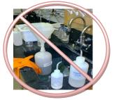
Hazardous waste must be accumulated in an area free of cracks and gaps ensuring containment and preventing release into the environment. Locating SAA's in a sink does not satisfy these criteria. To set up a proper SAA obtain a secondary containment bin in Cambridge visit the VWR Stockrooms basement of Naito and Biological Laboratories. In Longwood call 2-1720. Set up SAA at or near point of generation (NOT IN SINK).
