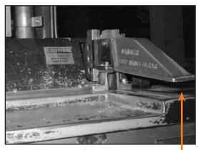
Missing "nose guard" on this jump saw.
