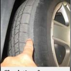
Check tires for proper tread wear, tire pressure and damage
