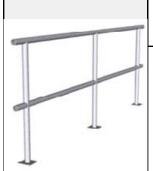
A standard guardrail must be 42 inches in height, have an intermediate rail, proper spacing of the posts and be capable of supporting 200 lbs of force
