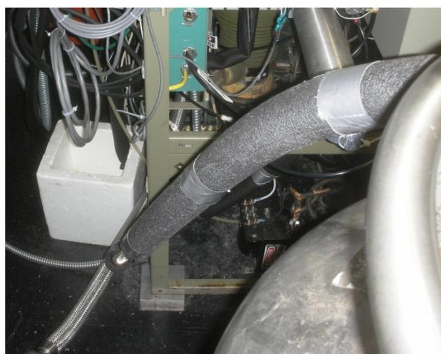
Figure 7 Container for LN2 overflow when filling cold trap. What happens if this becomes blocked?
