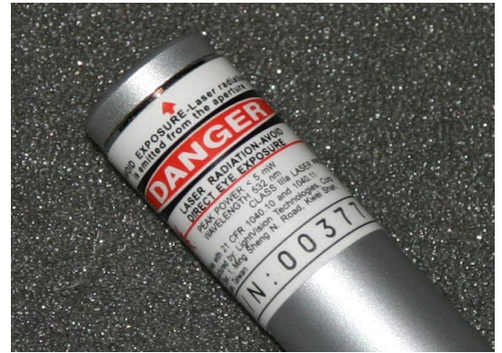
The warning label designs may not be the same. But the labels have to include: the starburst insignia, laser classification, maximum output power (in mW), and wavelength (in nm).
