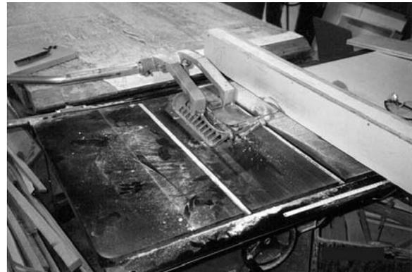
Table saw equipped with self-adjusting blade guard.
