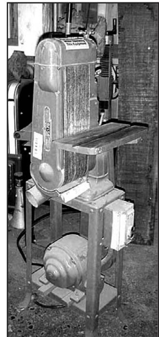
This vertical belt sander is equipped with guards on the sides to effectively cover the nip points created by the belt running onto the pulleys. Also, the work table is properly positioned close to the belt — minimizing the nip point created by the distance between the belt and table.
